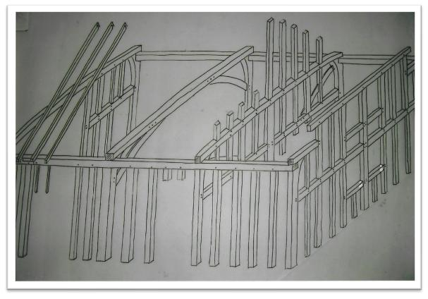
Pictured above: My drawing of the original timber frame, note gap in the front showing two studs missing, the doorway to the screens passage. Pictured inset: close up brickwork
